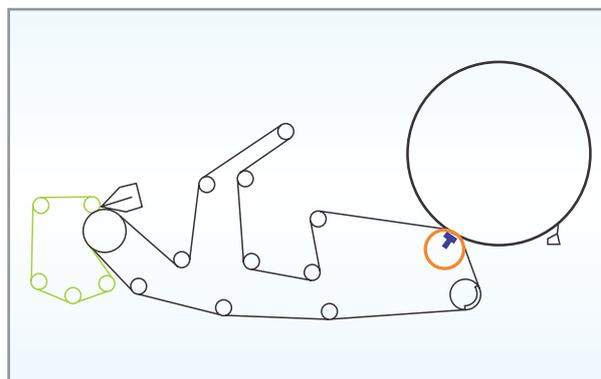
Figura 8: CrescentFormer (CF) + SR (suction roll) + shoe press (SP)
